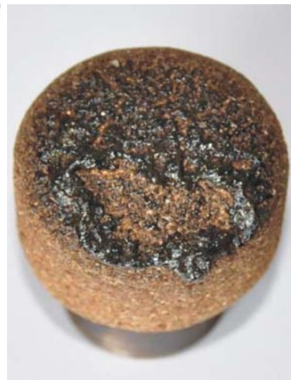
35 wt% tobermorite 65 wt% xonotlite
